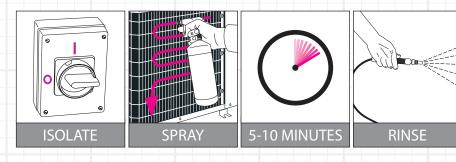
Isolate electrics. Spray into coil, starting at top corner and working methodically across and down. Rinse with fresh water.
