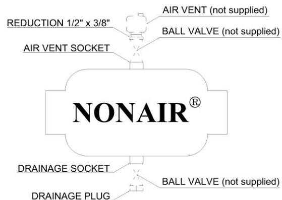
For drainage is at the bottom of NONAIR<sup>®</sup> a plugged 1/2", 3/4" or 1" female threaded socket dependent on size and type. For service of the drainage, unscrew the plug and mount a suitable ball valve in the socket.
