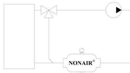
For Air outlet through an Air vent (not supplied from the factory) is on top of NONAIR<sup>®</sup>, depending on the size, 1 to 3 pcs of 1/2" female threaded sockets. For future service of the Air vent mount a 1/2" ball valve (male thread in/female thread out) in between. If the Air vent has 3/8" inlet mount the 1/2 x 3/8" reduction supplied between the ball valve and the Air vent.
