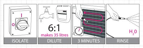
Isolate electrics. Dilution: use between 1 and 6 parts water, depending on contamination of coil. Start cleaning at bottom of coil and work methodically across and up. Cleaning is more effective if condenser is still warm. Wait 3 minutes or until foam action has stopped, then rinse thoroughly with fresh water.
