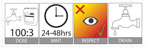
Wherever possible, clean all systems with compressor and pump working normally.
