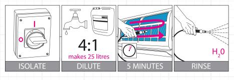
Dilution 1:4 parts water. Turn off unit and isolate electrics. Apply diluted CondenCide® with a low pressure sprayer set on a coarse spray pattern. Saturate areas to be cleaned and keep wet for 5 minutes. Contaminated CondenCide® will drain away as normal condensate. After cleaning, flush thoroughly with fresh water. Let surfaces air dry before re-starting system.
